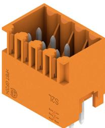
Straight, double-row pin header available in closed-sided or flange version (open-sided pin headers on request). The male headers with a pin length of 3.5mm are designed for wave soldering and are packed in a box. They can be screwed on to the PCB. The male headers provide space for labelling and can be coded.
