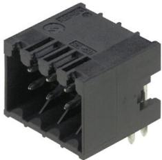
High-temperature-resistant, straight, 2-tier male connector for all common soldering methods. Optimised for automatic assembly. Packed in box or tape. 3.2 mm solder pin suitable for reflow and wave soldering. These male connectors can be labelled and coded.
