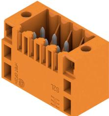
Straight, double-row pin header available in closed-sided or flange version (open-sided pin headers on request). The male headers with a pin length of 3.5mm are designed for wave soldering and are packed in a box. They can be screwed on to the PCB. The male headers provide space for labelling and can be coded.
