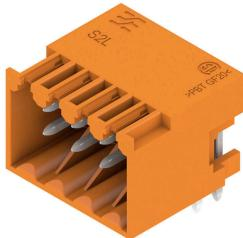
Angled, two-tier pin header available as closed-sided or with flange (open-sided pin headers on request). Pin headers with 3.5mm pins are designed for wave soldering and are packaged in a box. They can be screwed on to the PCB. The pin headers provide space for labelling and can be coded.
