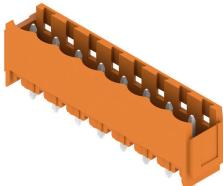
Pin headers in glass-fibre-reinforced plastic with straight wire outlet; optimised for wave soldering. The flange variant (F) can be screwed onto the respective counter piece or the circuit board. There is no need for an extra screw to connect the circuit board when the solder flange (LF) version is used. This also protects the solder points from mechanical strain. All pin headers can be manually coded or ordered pre-coded. HC = High Current.
