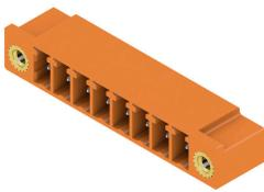
The SC pin header has a parallel (recumbent) plugging direction in relation to the PCB. It is available in closed (G) and screw flange (F) versions. Weidmüller's 3.81-mm-pitch (0.15 inch) plug-in connectors are compatible with the layouts of standard connectors. They support a flood-light display and offer space for labelling and coding.
