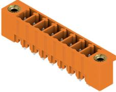
The SC pin header has a perpendicular (standing) plugging direction in relation to the PCB. It is available in closed (G) and screw flange (F) versions. Weidmüller's 3.81-mm-pitch (0.15 inch) plug-in connectors are compatible with the layouts of standard connectors and offer space for labelling and coding.
