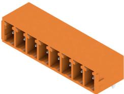
The SC pin header has a parallel (recumbent) plugging direction in relation to the PCB. It is available in closed (G) and screw flange (F) versions. Weidmüller's 3.81-mm-pitch (0.15 inch) plug-in connectors are compatible with the layouts of standard connectors. They support a flood-light display and offer space for labelling and coding.
