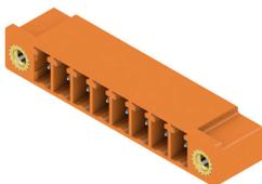
The SC pin header has a parallel (recumbent) plugging direction in relation to the PCB. It is available in closed (G) and screw flange (F) versions. Weidmüller's 3.81-mm-pitch (0.15 inch) plug-in connectors are compatible with the layouts of standard connectors. They support a flood-light display and offer space for labelling and coding.
