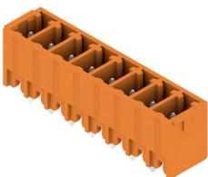
The SC pin header has a perpendicular (standing) plugging direction in relation to the PCB. It is available in closed (G) and screw flange (F) versions. Weidmüller's 3.81-mm-pitch (0.15 inch) plug-in connectors are compatible with the layouts of standard connectors and offer space for labelling and coding.
