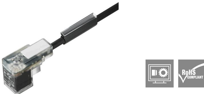
Weidmüller can supply valve plugs as connecting lines with M8/M12 plugs and one end without connector. The status of the valve plug is shown by an LED. The valve plugs have a protective circuit. The Weidmüller range includes valve plugs of type A, B and C to DIN and industry standards. Protection class IP 67 is fulfilled when screwed in. The outlet direction is also a decisive factor, therefore Weidmüller offers different versions.
