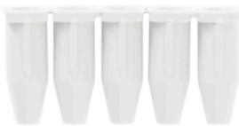
The use of reducing sleeves simplifies the connection of conductors with smaller cross-sections. Conductors can be reliably inserted into the clamping point without the strands fraying. The use of a reducing sleeve centres the conductor in the entry point.
