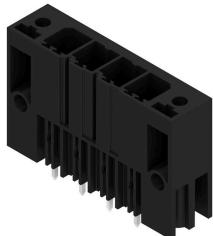
Single-row, high-performance male header for side-by-side mounting without sacrificing any poles or with patented flange for fast fixing without tools. Maximum connection and operating reliability thanks to a mating profile that prevents incorrect connection, with unique coding diversity and additional fastening in the flange. 3.5 mm pin length is optimised for lead-free wave soldering.
