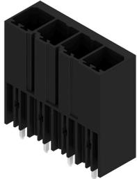
Single-row, high-performance male header for side-by-side mounting without sacrificing any poles or with patented flange for fast fixing without tools. Maximum connection and operating reliability thanks to a mating profile that prevents incorrect connection, with unique coding diversity and additional fastening in the flange. 3.5 mm pin length is optimised for lead-free wave soldering.
