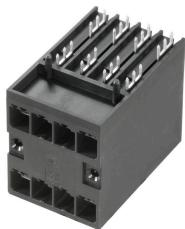
Double-row high-current, high-performance pin headers, with or without flange, for fast, tool-free locking. Optimised for "book-size modules" measuring 50mm wide and above. With integrated mounting option for mounting to the housing wall. Exceptional reliability and operational safety thanks to 100% failsafe mating profile, unique coding and optional additional screw mounting in the flange.
