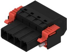
Inverted male header with PUSH-IN connection technology for field wiring with inverted external flanges in 6 mm<sup>2</sup> with a 7.62 pitch. Also ideal as a touch-safe solution for inverse voltages. Meets the requirements of UL1059 600 V class C and IEC 61800-5-1. Optionally also available as screwable version and without flange.
