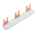
The distribution or multiplication of a potential to adjoining terminal blocks is realized via a cross-connection. Additional wiring effort can be easily avoided. Even if the poles are broken out, contact reliability in the terminal blocks is still ensured. Our portfolio offers pluggable and screwable cross-connection systems for modular terminal blocks.
