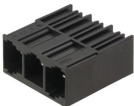
Single-row, high-current male header, for side-by-side mounting without sacrificing any poles, or with patented flange for fast locking without tools. Maximum connection and operating reliability thanks to a mating profile that prevents incorrect connection, with unique coding diversity and additional fastening in the flange. 3.5 mm pin length is optimised for wave soldering, plug-in direction 90° to solder pins.
