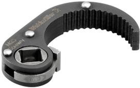
The Screwty® attachment is suitable for customisable M23 round plug-in connectors and for overmoulded M23 round plug-in connectors, with an outside dimension of the knurled nut of  $26.2 \pm 0.3$  mm. The tightening torque is 2-2.5 Nm.
