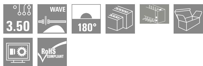
Double-level, staggered pin header for wave soldering at 3.50 mm pitch. They are available in closed and flanged versions. The male connectors provide space for labelling and can be coded.
