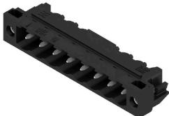
High-temperature-resistant pin header, packed in box or tape. On tape, with 1.5 mm solder pin, optimised for automatic assembly. 3.2 mm solder pin suitable for reflow and wave soldering. The pin headers provide space for labelling and can be coded. HC = High Current.
