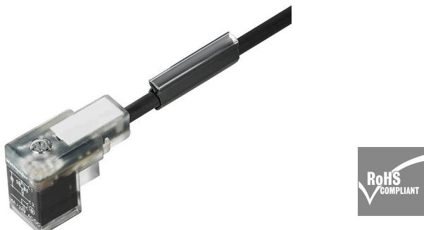
Weidmüller can supply valve plugs as connecting lines with M8/M12 plugs and one end without connector. The status of the valve plug is shown by an LED. The valve plugs have a protective circuit. The Weidmüller range includes valve plugs of type A, B and C to DIN and industry standards. Protection class IP 67 is fulfilled when screwed in. The outlet direction is also a decisive factor, therefore Weidmüller offers different versions.
