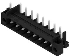
High-temperature-resistant, straight, open pin header. Packed in box or tape. On tape and with 1.5 mm solder pin, optimised for automatic assembly. 3.2 mm solder pin suitable for reflow and wave soldering. The pin headers provide space for labelling and can be coded. HC = High Current.
