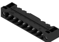
High-temperature-resistant pin header, packed in box or tape. On tape, with 1.5 mm solder pin, optimised for automatic assembly. 3.2 mm solder pin suitable for reflow and wave soldering. The pin headers provide space for labelling and can be coded. HC = High Current.
