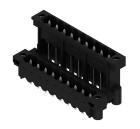
High-temperature resistant, double level, laterally offset, male connector with flange or solder flange. 1.5 mm solder pin is suitable for reflow soldering. 3.2 mm solder pin suitable for reflow and wave soldering. The pin headers provide space for labelling and can be coded.
