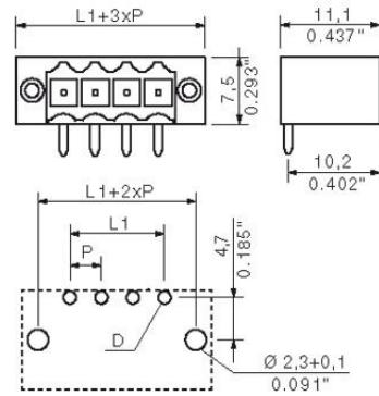
$L1 = 7.00 \text{ mm}$  |  $P = 3.50 \text{ mm}$
