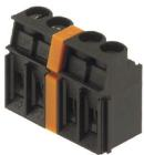
The maximum voltage is based on the minimum distance. Intermediate plates increase the creepage and clearance distances between different potentials and permit higher rated voltages or a clear separation, e.g. between mains and low voltages or different protection zones.
