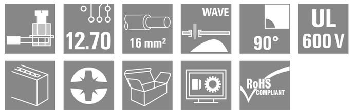
This PCB terminal provides connections for 1000 V, 76 A and 16 mm<sup>2</sup> conductor cross-section with proven clamping yoke connection at 12.7 mm pitch, conductor outlet direction in 90° design.
