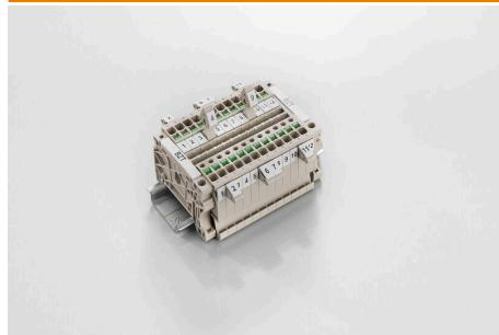
The marker holder offer the possibility of additional mounting of standard markers with a pitch of 5 or 5.1 mm. The angled holders can be optionally snapped together and could be mounted in all standard marking channels of the Klippon® Connect modular terminal blocks. Fitting marker types could be found under the respective accessories of the designation marking holder.
