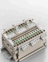
The marker holder offer the possibility of additional mounting of standard markers with a pitch of 5 or 5.1 mm. The angled holders can be optionally snapped together and could be mounted in all standard marking channels of the Klippon® Connect modular terminal blocks. Fitting marker types could be found under the respective accessories of the designation marking holder.
