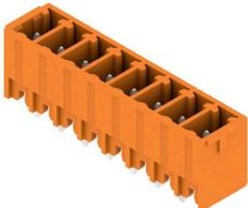
The SC pin header has a perpendicular (standing) plugging direction in relation to the PCB. It is available in closed (G) and screw flange (F) versions. Weidmüller's 3.81-mm-pitch (0.15 inch) plug-in connectors are compatible with the layouts of standard connectors and offer space for labelling and coding.
