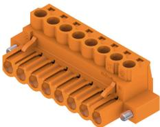
Female plug with clamping-yoke screw system for connecting wires with straight (180°) outlet direction. The female connectors provide space for labelling and can be coded. Fastened by means of a flange or release latch. They also provide an integrated plus/minus screw, protection against faulty insertion of the wire, and they are delivered with open clamping yokes. HC = High Current.
