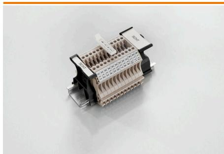
The SchT 5 S group tag carriers are clipped directly onto the TS 32 mounting rail (G-rail) or the TS 35 mounting rail (top-hat rail). It is therefore possible to label the terminal strip irrespective of the terminal and the type of terminal. SchT 5 and SchT 5 S are fitted with ESO 5, STR 5 protective strips.
