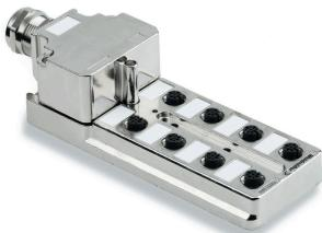
Some applications require complete shielding from the sensor to the control. Our metal SAI distributors achieve this complete shielding. EMC glands are included with the distributors. Initiator LEDs are omitted. They are available in 4- and 8-way M12 versions with 5 or 10 m cables. In addition, these distributors can be used in harsh environments e.g. in the vicinity of welding plant. Hoods with a generous connection space available so that they can be provided with a standard gland up to M25.
