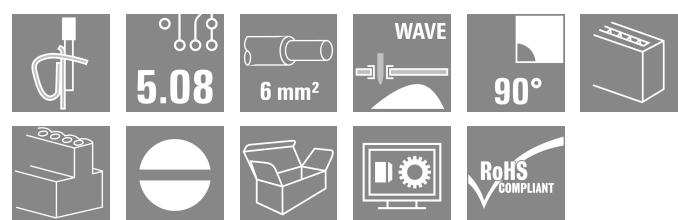
Disconnect element with test point, PCB terminal with proven clamping yoke connection at 5.08 mm pitch, conductor outlet direction 90°. Suitable for conductor cross-sections up to 6.0 mm<sup>2</sup>.
