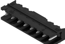
High-temperature-resistant, 90° angled, open male header. Packed in box or tape. On tape, with 1.5 mm solder pin, optimised for automatic assembly. 3.2 mm solder pin suitable for reflow and wave soldering. The pin headers provide space for labelling and can be coded. HC = High Current.
