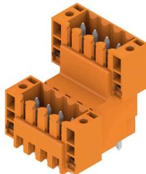
Double-level, staggered pin header for wave soldering at 3.50 mm pitch. They are available in closed and flanged versions. The male connectors provide space for labelling and can be coded.
