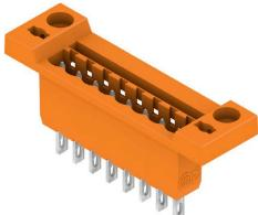
Male connector for through-panel mounting with optional locking function. Internal connection as flat-blade or solder connection. These male connectors provide space for labelling and can be coded.
