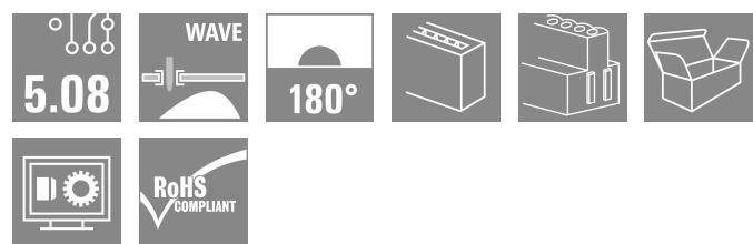
Female header for PCB mounting. The solder pin length is optimised for wave flow soldering.
