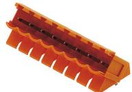
Male connectors with 135° outlet direction. The solder pin length is optimised for wave flow soldering. The pin headers provide space for labelling and can be coded.
