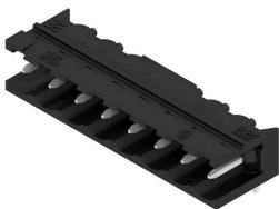
High-temperature-resistant, 90° angled, open male header. Packed in box or tape. On tape, with 1.5 mm solder pin, optimised for automatic assembly. 3.2 mm solder pin suitable for reflow and wave soldering. The pin headers provide space for labelling and can be coded. HC = High Current.
