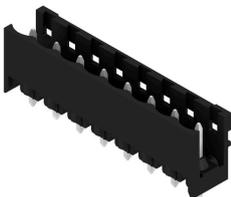
High-temperature-resistant, straight, open pin header. Packed in box or tape. On tape and with 1.5 mm solder pin, optimised for automatic assembly. 3.2 mm solder pin suitable for reflow and wave soldering. The pin headers provide space for labelling and can be coded. HC = High Current.
