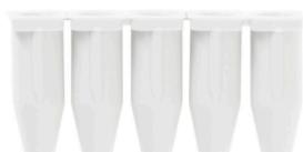
The use of reducing sleeves simplifies the connection of conductors with smaller cross-sections. Conductors can be reliably inserted into the clamping point without the strands fraying. The use of a reducing sleeve centres the conductor in the entry point.
