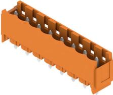
Pin headers in glass-fibre-reinforced plastic with straight wire outlet; optimised for wave soldering. The flange variant (F) can be screwed onto the respective counter piece or the circuit board. There is no need for an extra screw to connect the circuit board when the solder flange (LF) version is used. This also protects the solder points from mechanical strain. All pin headers can be manually coded or ordered pre-coded. HC = High Current.
