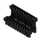
High-temperature resistant, double level, laterally offset, male connector with flange or solder flange. 1.5 mm solder pin is suitable for reflow soldering. 3.2 mm solder pin suitable for reflow and wave soldering. The pin headers provide space for labelling and can be coded.
