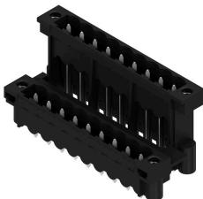
High-temperature resistant, double level, laterally offset, male connector with flange or solder flange. 1.5 mm solder pin is suitable for reflow soldering. 3.2 mm solder pin suitable for reflow and wave soldering. The pin headers provide space for labelling and can be coded.
