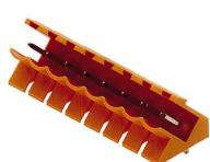
Male connectors with 135° outlet direction. The solder pin length is optimised for wave flow soldering. The pin headers provide space for labelling and can be coded.
