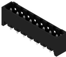
High-temperature-resistant pin header, packed in box or tape. On tape, with 1.5 mm solder pin, optimised for automatic assembly. 3.2 mm solder pin suitable for reflow and wave soldering. The pin headers provide space for labelling and can be coded. HC = High Current.
