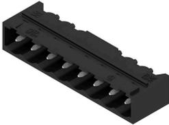
High-temperature-resistant pin header, packed in box or tape. On tape, with 1.5 mm solder pin, optimised for automatic assembly. 3.2 mm solder pin suitable for reflow and wave soldering. The pin headers provide space for labelling and can be coded. HC = High Current.
