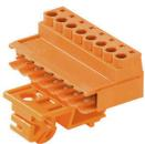
Male plugs with clamping-yoke screw wire-connect system. With clip-on feet for attaching the male plugs on rail. The male plugs provide space for labelling and can be coded.
