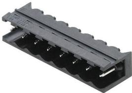
High-temperature-resistant, straight, open pin header. Packed in box or tape. On tape and with 1.5 mm solder pin, optimised for automatic assembly. 3.2 mm solder pin suitable for reflow and wave soldering. The pin headers provide space for labelling and can be coded. HC = High Current.
