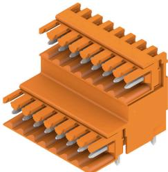
Double-level, staggered pin header for wave soldering at 3.50 mm pitch. They are available in closed and flanged versions. The male connectors provide space for labelling and can be coded.
