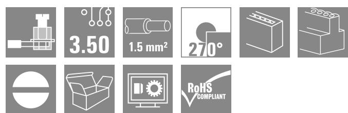
Female connectors with clamping yoke screw system for connecting conductors at 3.50 mm pitch. They provide space for labelling and can be coded.
