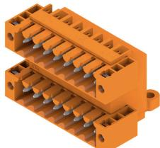
Two-tier pin header for wave soldering in 3.50 mm pitch. The connector is available in open, closed and flange versions. The male connectors provide space for labelling and can be coded. Packed in a cardboard box.
